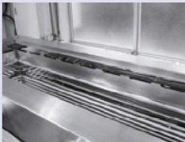
Increasing volume of cooling coil in order to raise free board ratio
