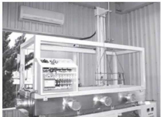
Transport equipment with model cleaning equipment for quantitative measurement experiment
